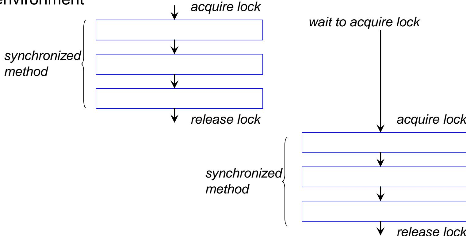
If one thread invokes a synchronized method on an object, **the lock of that object** is first acquired, the method body executed, and then the lock released. Another thread invoking a synchronized method **on that same object** will block until the lock is released
